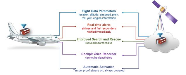
When triggered by distress conditions, the system will include flight data from a specified period of time preceding the incident and continue to download CVR/FDR data throughout the flight to aid investigators in understanding both what was happening during the distress period as well as the circumstances that led to it.
